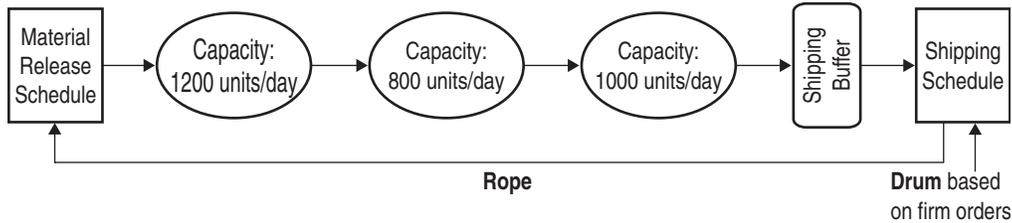
**FIGURE 3. THE SIMPLIFIED DRUM-BUFFER-ROPE MODEL**
