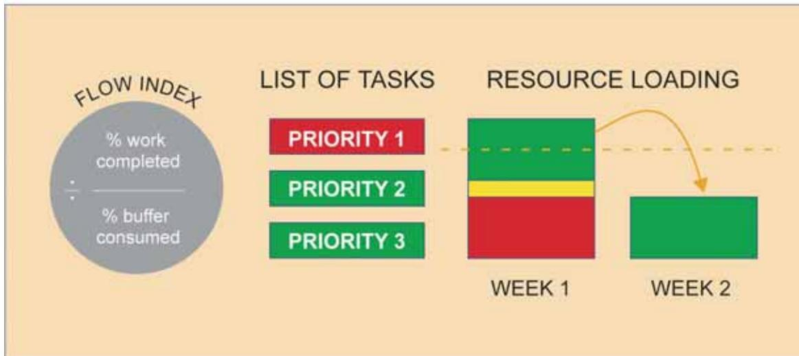
Fig. 3. Buffer Management. Drive execution priorities based on relative buffer consumption.
